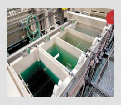
Electroless nickel plating is a chemical process that deposits a nickel-phosphorus alloy onto a substrate without using an electric current, resulting in a uniform, corrosion-resistant, and wear-resistant coating.
