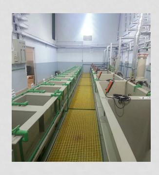
Zinc plating (also known as electro-galvanising) is a process where zinc is applied by using a current of electricity. Zinc plating involves the electrodeposition of a thin coating of zinc metal onto the surface of another metal object, known as a substrate.
